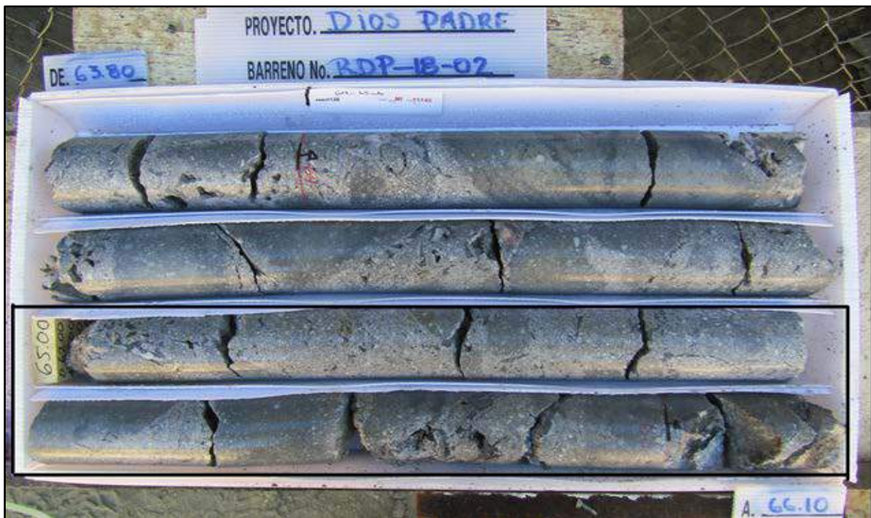
RDP 18-02 63.8 – 66.1 m, 931 g Ag Breccia 1,2 - primary and secondary breccia in andesite, note open vugs.
