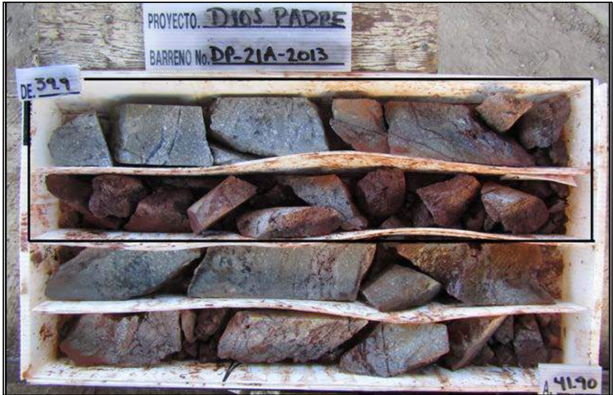
DP 21A -2013 39.5 – 41.9 m, 780 g Ag Breccia 1- stockwork, micro-fractures in rhyolite, note re-healed textures.
