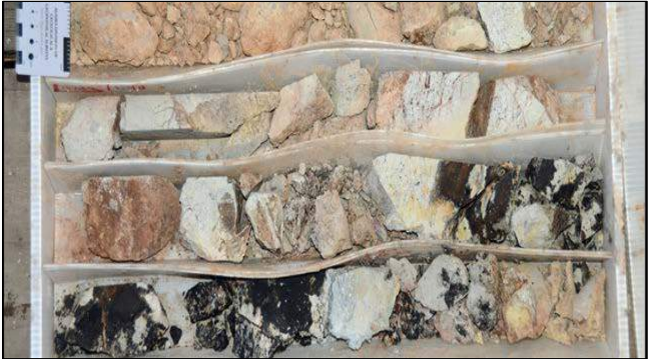
DPD 26 -2013 106 – 108 m, 1000 g Ag Fault 1 - fault gouge in rhyolite.
