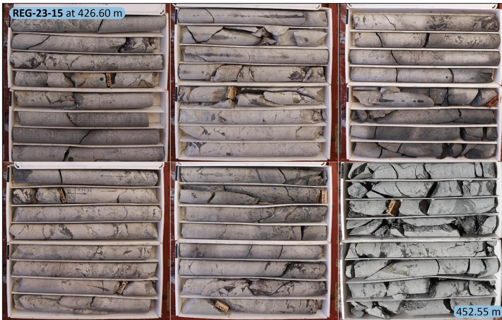
Figure 3b: REG-23-15 - Mineralized specularite-pyrite-chalcopyrite breccia from 426.6m - 452.55
