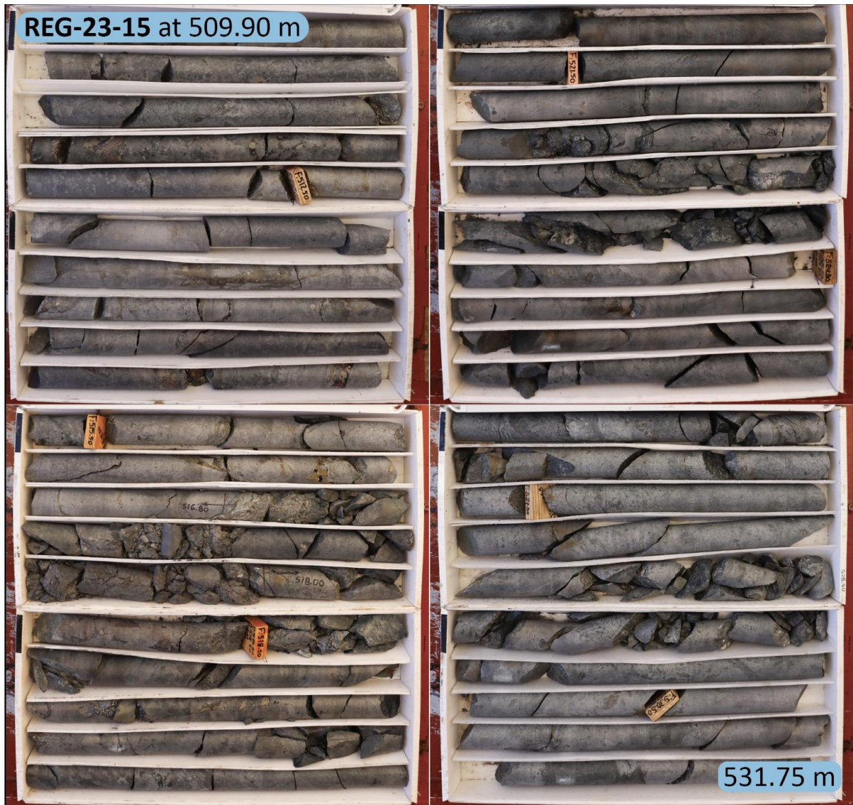
Figure 3e: REG-23-15 - Mineralized specularite-pyrite-chalcopyrite breccia from 509.90m – 531.75m
