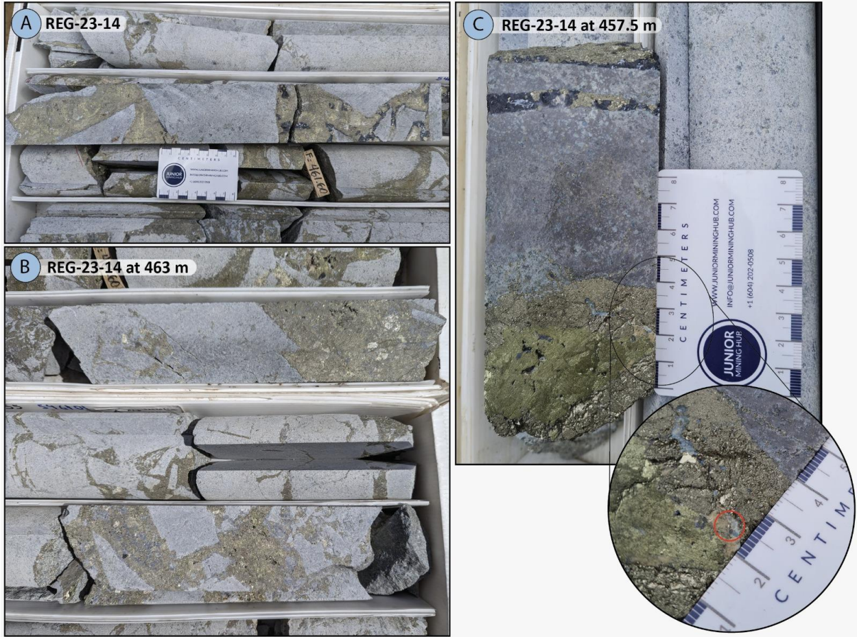
Figure 4: REG-23-14 – Strongly pyrite-chalcopyrite-specularite mineralized zones within broad breccia intersection. C shows a small flake of visible gold adjacent to the sulphides.
