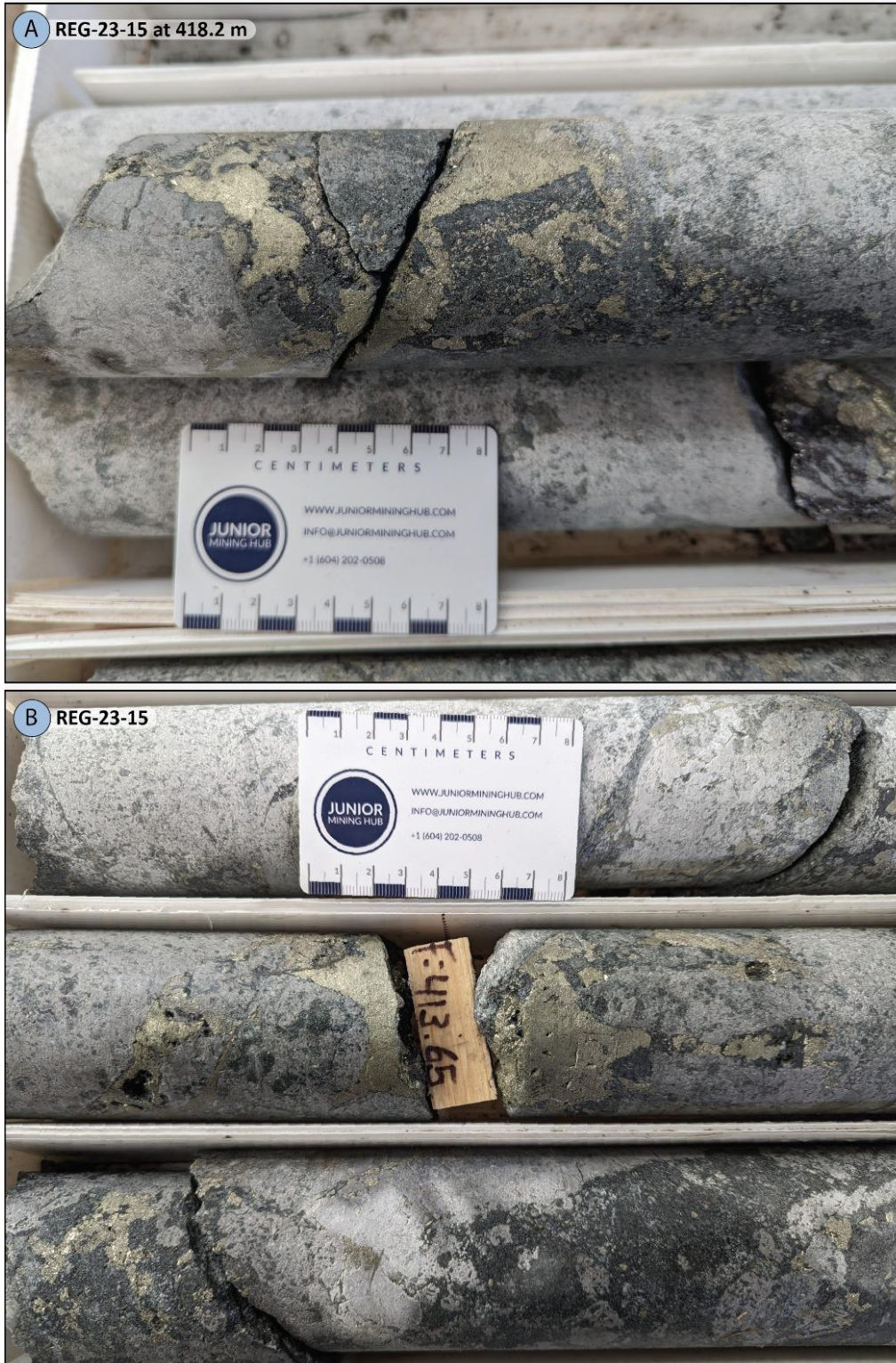
Figure 5: REG-23-15 – Strong specularite-pyrite-chalcopyrite mineralized zones within broad breccia intersection.
