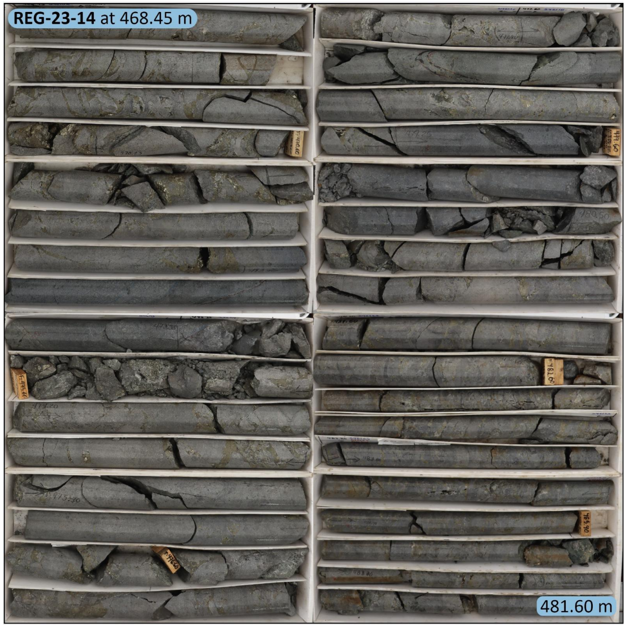
Figure 2b: REG-23-14 - Mineralized pyrite-specularite-chalcopyrite breccia from 468.45m-481.6.
