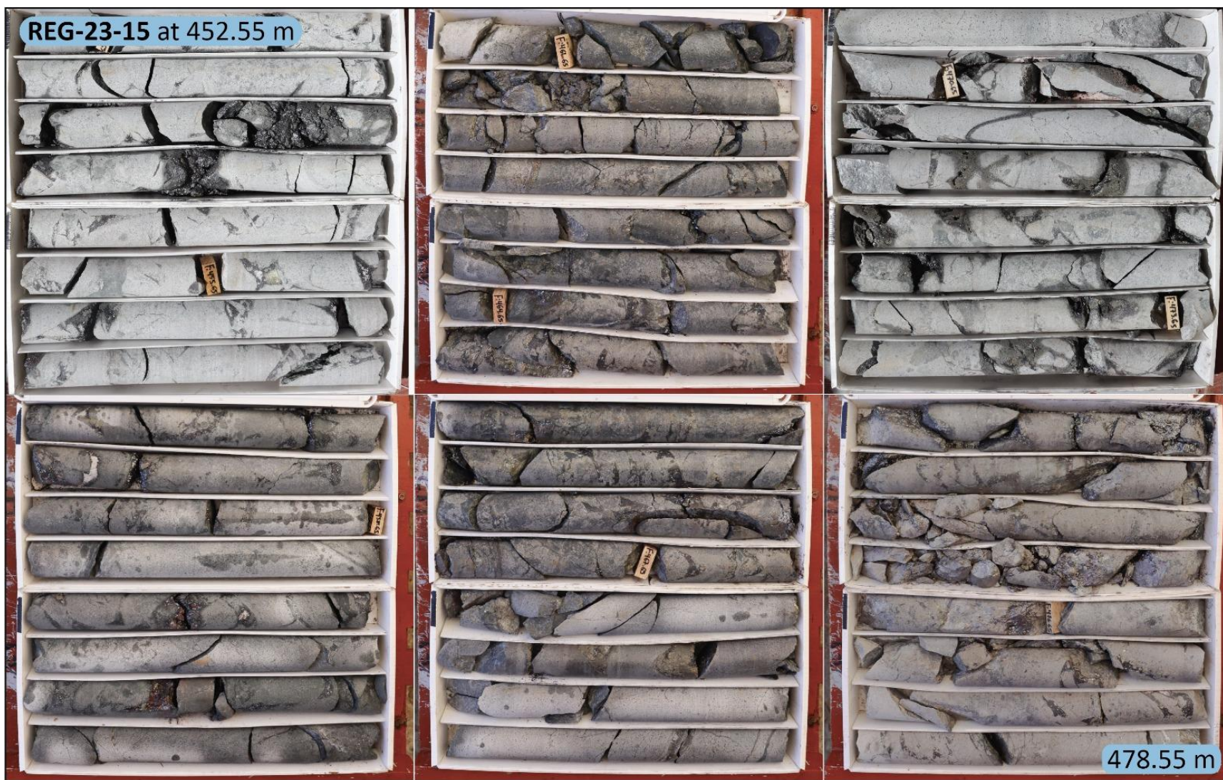
Figure 3c: REG-23-15 - Mineralized specularite-pyrite-chalcopyrite breccia from 452.55m – 478.55m
