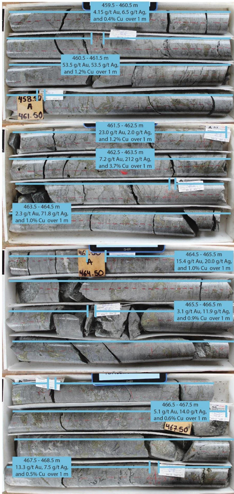
Figure 6: REG-22-01 - Mineralized specularite-pyrite-chalcopyrite breccia from 459.5m - 468.5m with assay results labelled.
