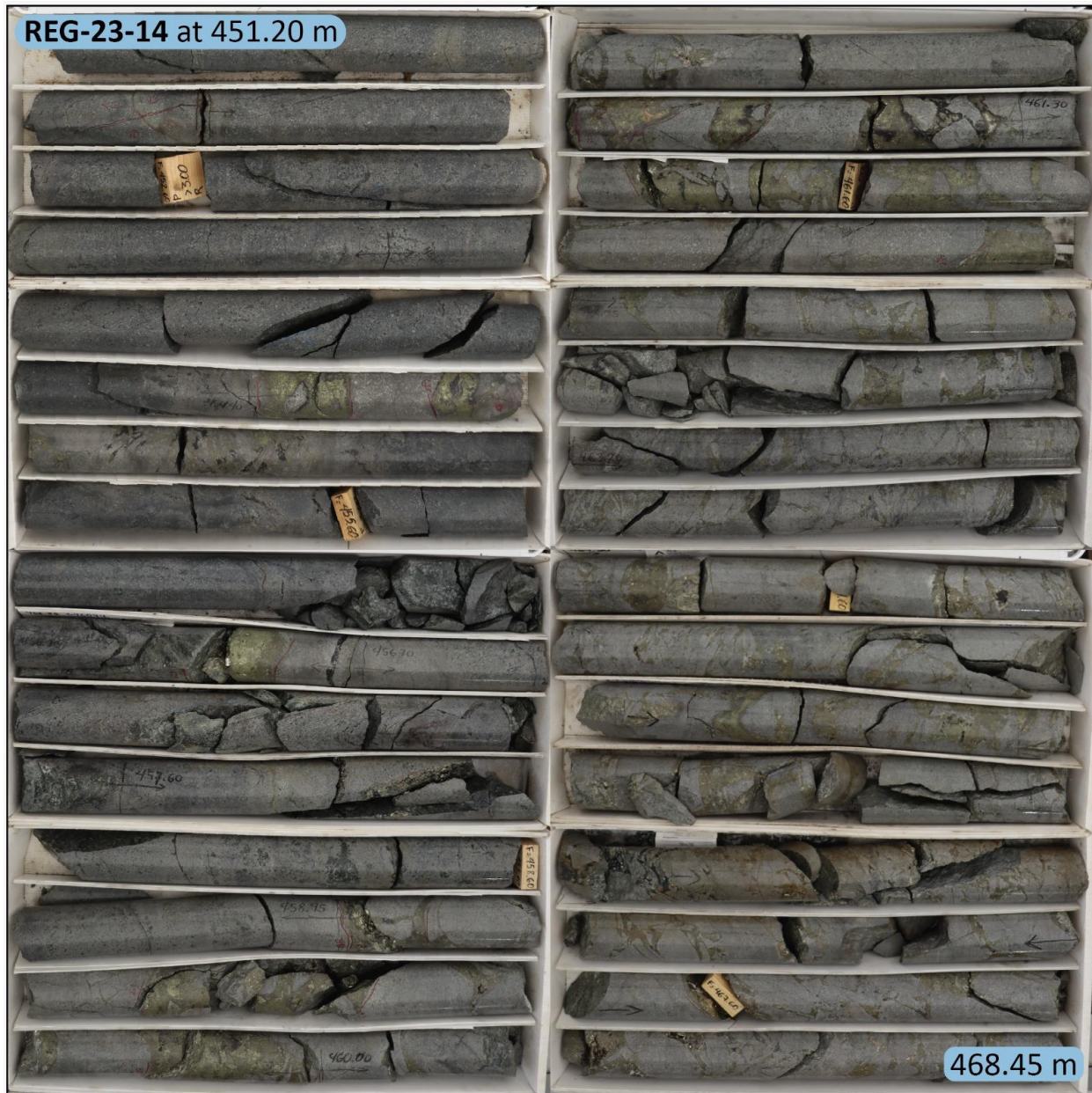
Figure 2a: REG-23-14 - Mineralized pyrite-specularite-chalcopyrite breccia from 451.2m – 468.45m.
